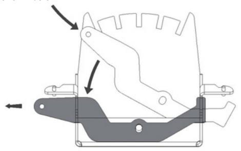
Reinstall the pivot head with the pivot head pin passing through the holes in the front cylinder mounting brackets (Item 2). Bolt on the two rear cylinder mounting brackets (Item 3). Attach the hydraulic cyclinder (Item 1) using the clevis
